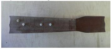
Install the frets into the frets slots. Clip the fret wire to length and press or tap into the slots. Tip: brush a small amount of water into the fret slots to soften the wood fibers before pressing in the frets.
