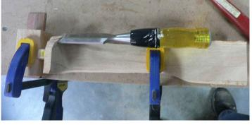
I use chisels for rough shaping, then progress to the belt sander, then hand shaping with flexible shaft tool, files and scrapers.
