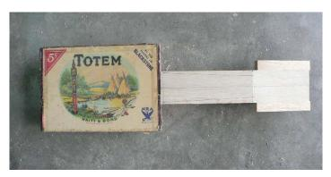
Lay the top on the body, and mark where the Bridge and sound hole will be.
